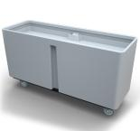
**Overview:** This ergonomic and worker-friendly feed cart was designed to fit comfortably underneath the ironer feed board for easy access to linen. The 28P16 is slightly longer and narrower than the 28P18 to accommodate wider ironers and remain conveniently placed under the feed board. The coil spring platform rises as items are removed, making it easier for team members to access linen. This promotes productivity and
